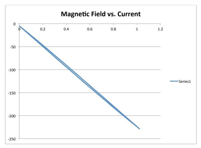
Appendix C: Preliminary Data for Characterizing the Quadruple magnets
